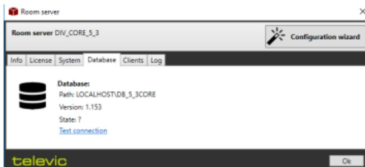
Figure 1-2 Where to find the SQL database name in the CoCon Room Server
